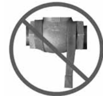
C.) Incorrect Installation: Heating tape hanging free from the surface
