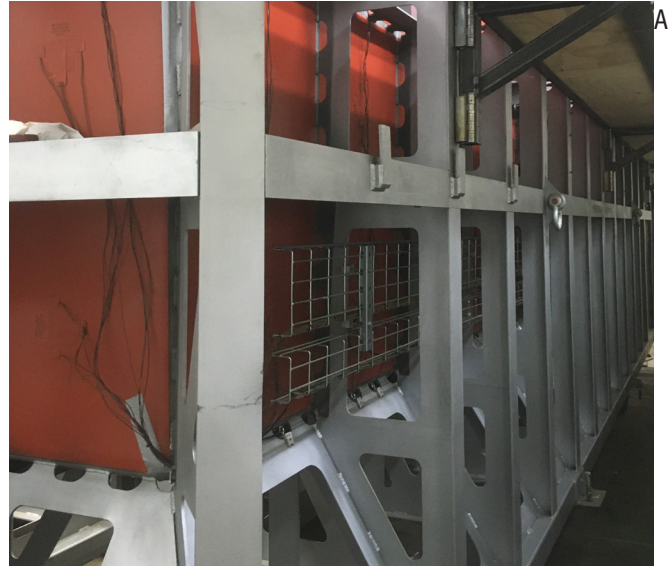
Figure 4- Heating blankets secured to mold (Courtesy of BriskHeat Corporation)
