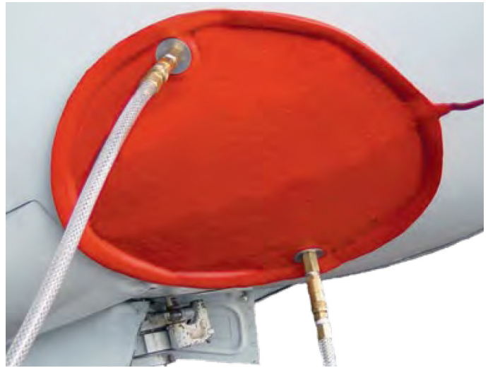
Figure 5- Combination reusable heater with vacuum capability (Courtesy of BriskHeat)
