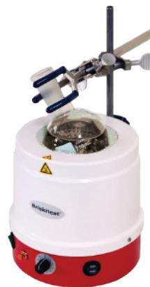
HM Metal Housed Heating Mantle
