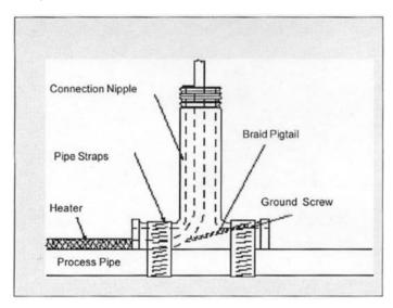
6. Connect the lead wires to the screws on the light fixture. Fill the connection nipple with the silicone sealant. Stow any excess lead wire in the box and mount the light fixture into the box. Attach the box cover to the box and attach the caution label to the cover. For those covers which have two mounting holes that are not used for the light assembly, place a small amount of silicone into and over the holes to seal out any moisture.
