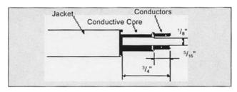
b. Strip 5/16" of insulation from each lead wire and connect a lead wire to each of the heater conductors using the insulated butt connectors. Wrap each connection and heater conductor with the silicone self-fusing tape, making sure to completely cover all exposed black core material and to overlap the heater jacket. Wrap over the self-fusing tape with fiberglass tape.
