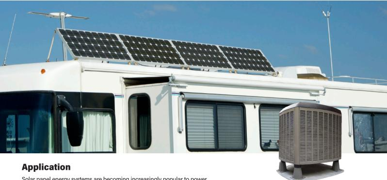
Solar panel energy systems are becoming increasingly popular to power homes, RVs, boats and more. There are also a huge number of aftermarket kits containing the basic components: solar panels, charge controllers, batteries, and inverters. These kits are rated based on the wattage that can be supplied by the panels and the amp hours that can be stored in the battery bank.
