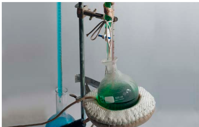
Heating mantle and flexible heating tape installed in a laboratory
