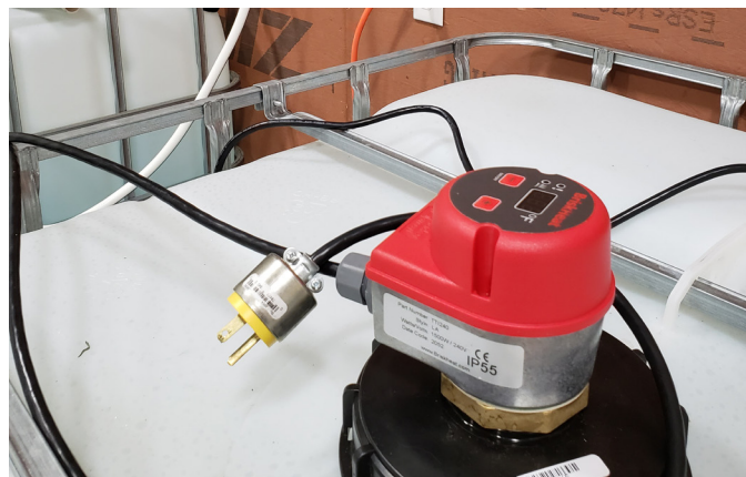
Immersion heater installed on IBC/Tote Tank
