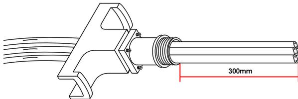
2. Lightly cut around cable jacket 165mm from the end of cable. Bend cable to break jacket. Lightly cut the jacket up the center between the first cut mark and the end of cable. Bend cable to break jacket. Remove the jacket from the heating cable.
