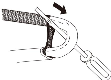
5. Lightly cut around cable insulation 145mm from the end of cable. Bend cable to break the insulation. Lightly cut the insulation up the center between the first cut mark and the end of cable. Bend cable to break jacket. Remove the insulation.
