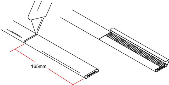
3. Move braid back toward the overjacket, creating a bulge. At the bulge, separate the braid to make an opening.
