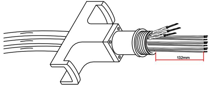
13. Insert the cables through the lower entry of the junction box.
