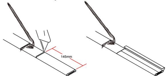
6. Shave off out matrix material from each bus wires with a utility knife.
