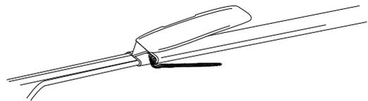
7. Peel back exposed wires from central matrix. DO NOT CUT THE BUS WIRES.
