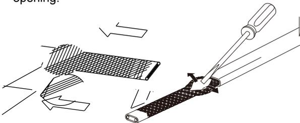
4. While bending the heating cable, work it through the braid opening. Pull the braid tight.
