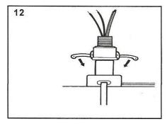
Slide the top in place and push and lock the cam levers into position. Lock cam levers by inserting the nylon zip tie wire through the holes in the ends of the cam levers and twisting together, inserting nylon zip tie through holes in the ends of the cam levers and pull tight to secure.
