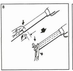
Cut inner core at end as shown. Roll back with pliers and peel bus wires away from core.
