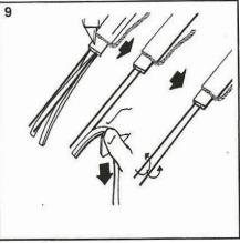
Remove core material from between the bus wires and any core material remaining on the bus wires
