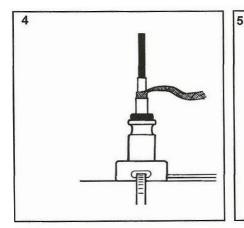
Strip the inner jacket 6" from the end. Strip the bus wires out of the core, following the Heat Trace Stripping Instructions.
