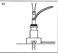
Start sliding the bus wires into the clear tubes (these function as guide tubes) that are inside the termination boot.
