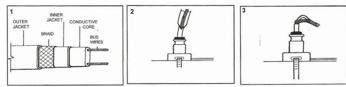
Extend the heater 7  $\frac{1}{2}$ " above the base. Slide the grommet over the heater inserting the grommet in the base. Strip outer jacket 7" from end. Attach the base to the pipe with a pipe strap.
