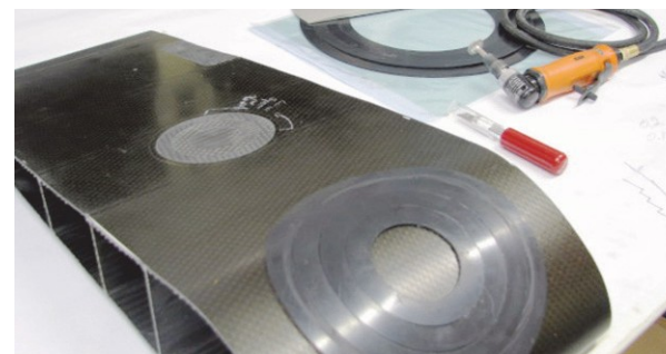
Figure 3: Illustration of routing, scarfing and stepping operations
