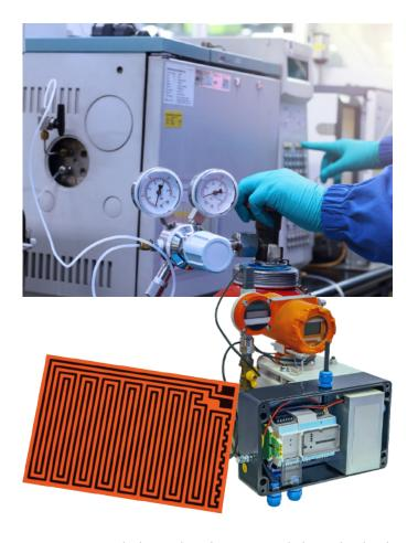
Hot/wet gas analysis requires the gas sample be maintained above the dewpoint temperature. Heating probes and sensing lines prevent condensation of liquid and maintain particulates in suspension. Analyzers designed to work with hot/wet samples typically require temperatures of approximately 302°F (150°C). Etched foil heaters are perfect for analysis requiring heated gas.
