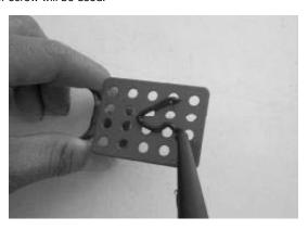
4. Spread sealant on top of nail or screw heads.
