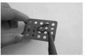
4. Place clip on prepared surface. Press down to ensure adhesive flows through holes.
