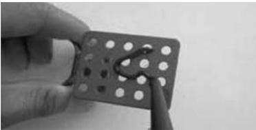
4. Orient the clip as needed on the roof. Place the roof clip on the roof where the roof is marked. Press down on the clip so that the adhesive flows through the holes. The cable insertion clamp should be vertical on the roof.
