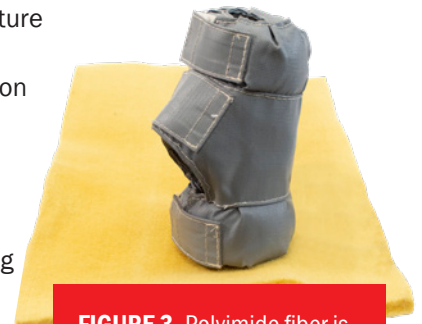
FIGURE 3. Polyimide fiber is a more durable alternative to fiberglass.
